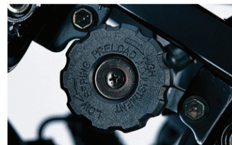
Useful rear spring preload adjustment
