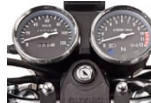
Large, clear speedo, tachometer and gear-position indicator
