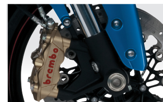
Radial mount Brembo monobloc calipers
